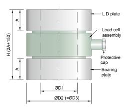
5000, 7500 kN and 10,000 kN load cell
